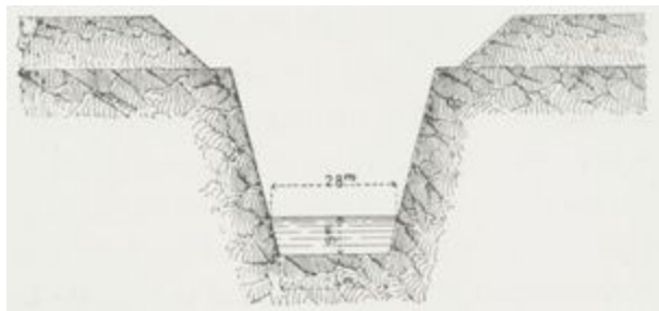
Fig. 13. — Profil du canal interocéanique dans les roches. The diagram shows a cross-section of a canal cut into hard rock. The water level is indicated by a horizontal line. The width of the waterway at the water level is marked as 28m. The sides of the canal are steep and vertical, contrasting with the sloping sides in Fig. 12. Above the water level, there are horizontal lines representing embankments or banquettes.
